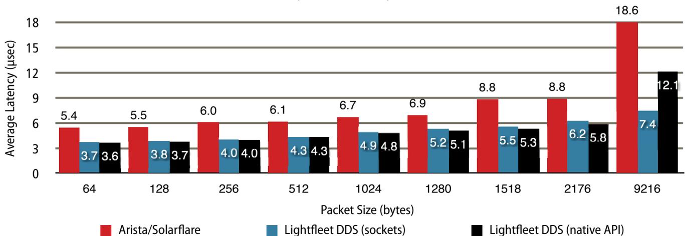
Notes: 1) Arista 7150S-52 switch was run in cut-through mode, 2) Arista 7150/Solarflare 7122 NIC latency measured with sockperf network benchmark tool (ping-pong) using UDP protocol 3) Lightfleet DDS latency with sockets measured with sockperf and libsockl, 4) Lightfleet DDS latency with native API measured using ping-pong. Packet sizes/methodology per RFC 2544 5) Latencies of optical transceivers and fiber cables are included in latency results.
